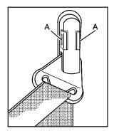
To move it up or down, squeeze the release buttons (A) together and move the height adjuster to the desired position.
